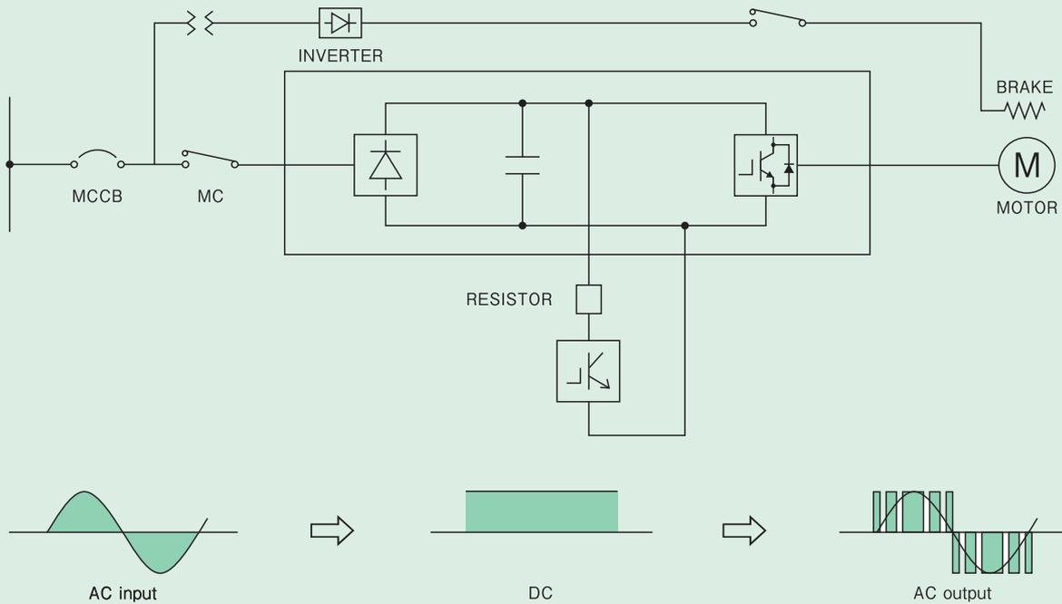
The control panel consists of inverter unit, transistor for regenerative braking, and circuit for magnetic brake.
